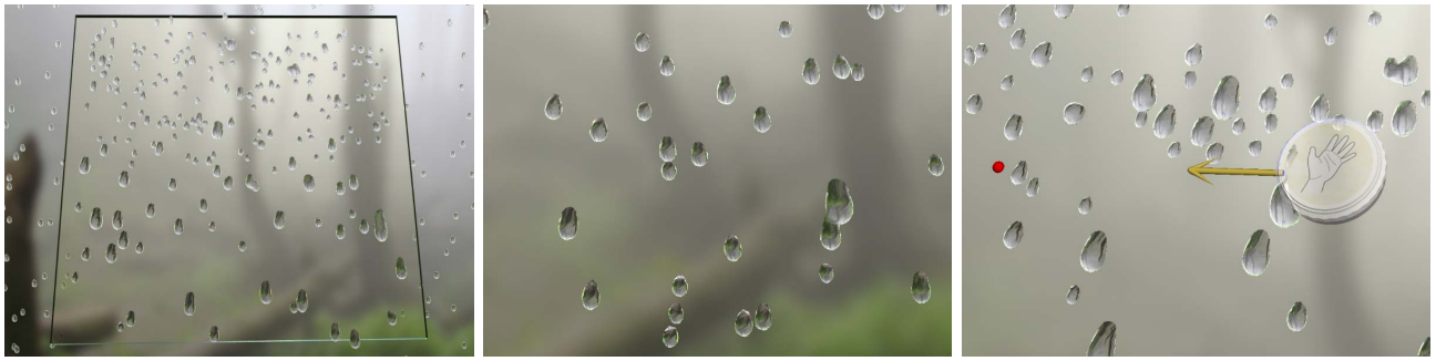
Fig. 10: Hundreds of droplets flowing on a window panel. The advancing contact angle is 90^\circ and the receding contact angle is 30^\circ . These images are taken from an interactive demo.
