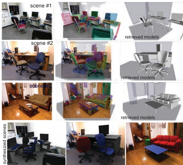
Figure 18: Based on single view RGBD scans (left), our algorithm extracts a set of stable arrangement of cuboids (middle). The arrangement is then used to retrieve matching 3D meshes with cuboid decomposition and used for scene modeling (right). (Bottom row) Retrieved models can be repositioned, rendered, and combined with the original RGB to synthesize novel manipulated images.
