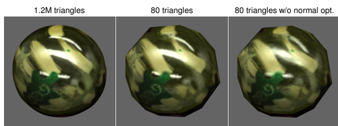
Fig. 11. Impact of geometric model error. We perform our joint optimization on the simplified geometry with (center image) and without the normal optimization (right image).
