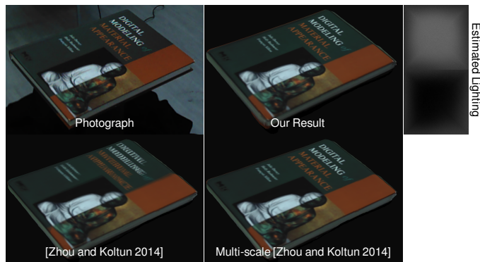
Fig. 7. Comparisons between our method and previous work on the diffuse Book model. We estimate both the SVBRDF and lighting, while [3] computes textures only. Note that the top-left photograph is not used in material/lighting/normal optimization.
