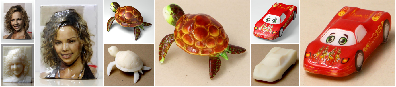
Fig. 13. Colored 3D prints produced using our method. The upper left image next to each model is the rendering result and the lower left image shows the model produced by 3D printing before coloring.
