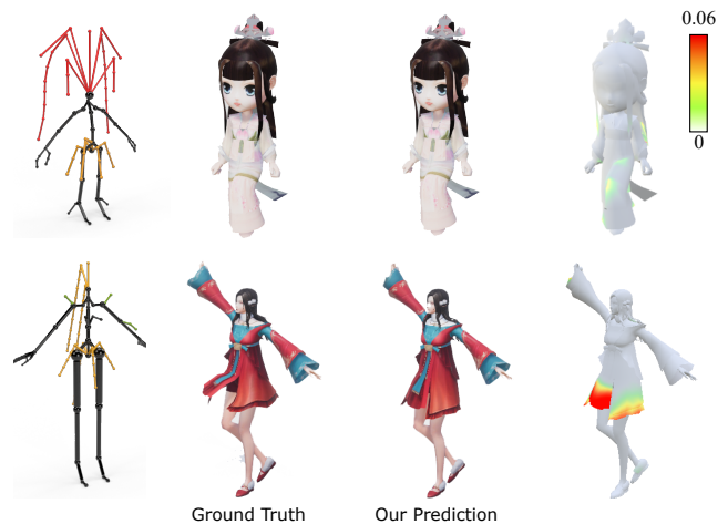
Fig. 9. Skin binding for characters that have skeleton structures not covered in the training set. Notice that the character in the bottom row shows larger prediction errors, mainly due to the incorrect binding of the skirt to the leg bone.
