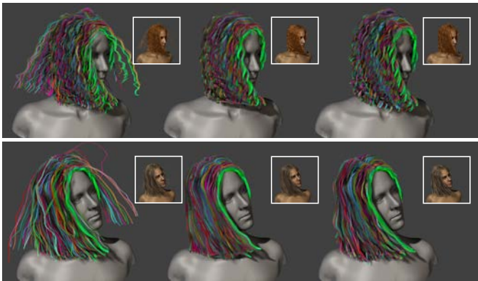
Fig. 17: Comparison to the State-Of-The-Art on Multiple Hairstyles. From left to right: Chai et al. [10], our method, and the ground-truth. Results of [10] have artifacts on both training data (top row) and test data (bottom row).
