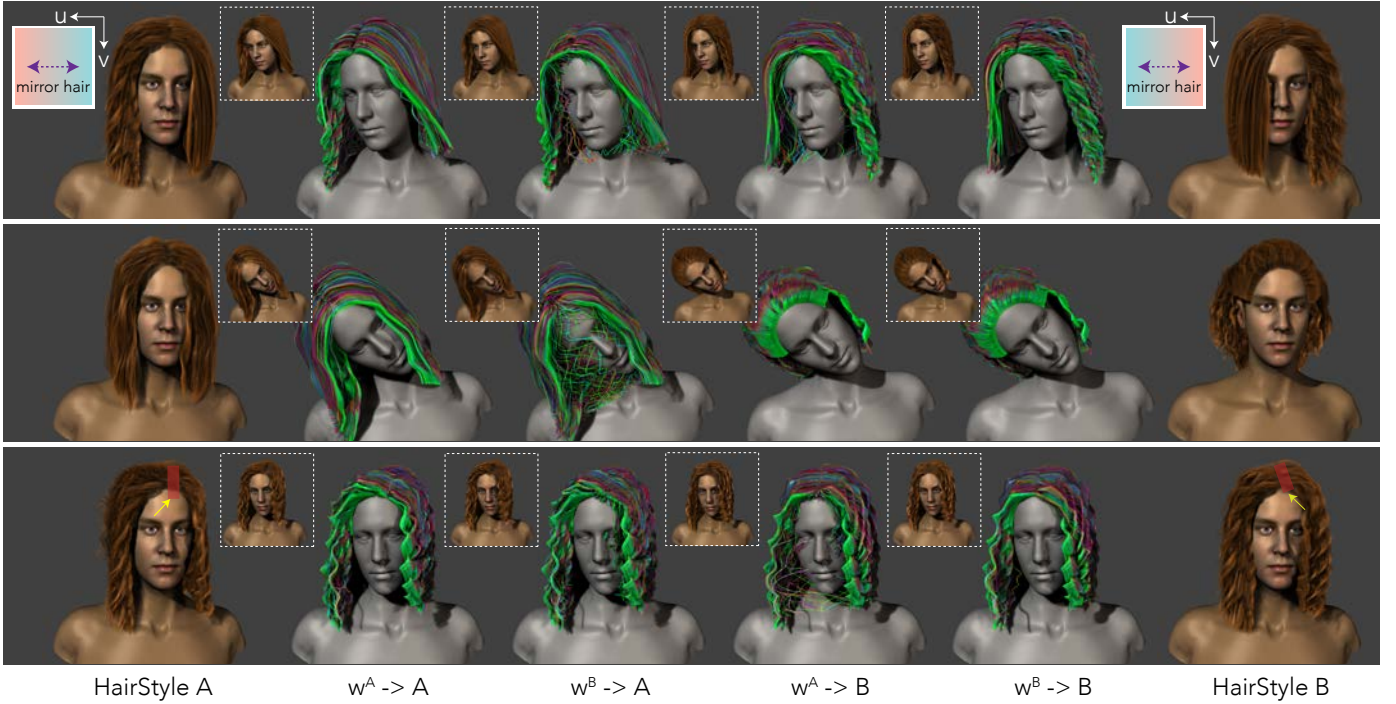
Fig. 11: Generalization. Our method produces reasonable weights according to different hairstyles that vary in factors like distributions (top row), growth directions (middle row), and parting styles (bottom row). Swapping the weights of hairstyle A (leftmost column) and hairstyle B (rightmost column) for interpolation leads to severe artifacts (the two columns in the middle). This observation proves the adaptability of our neural interpolator.
