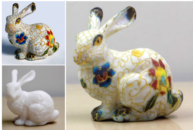
Figure 1: Colorful Bunny. We present a new computational approach for hydrographically printing arbitrary color textures on complex 3D surfaces and aligning the textures precisely. The input of our system includes the desired surface texture (upper left) of a physical shape (lower left). Through our hydrographic system, we color the surface of the 3D shape using the desired texture (right).
